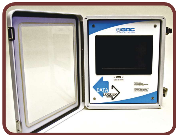
The Datalogger-4200 is a high-performance surface monitoring and automation system designed to interface with Sercel-GRC's digital downhole sensors. (Photo courtesy of Sercel-GRC)
