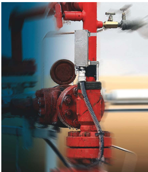
ETC's Sasquatch plunger velocity sensor is used to measure the surface velocity of a plunger before the impact at surface. (Photo courtesy of Extreme Telematics Corp.)
