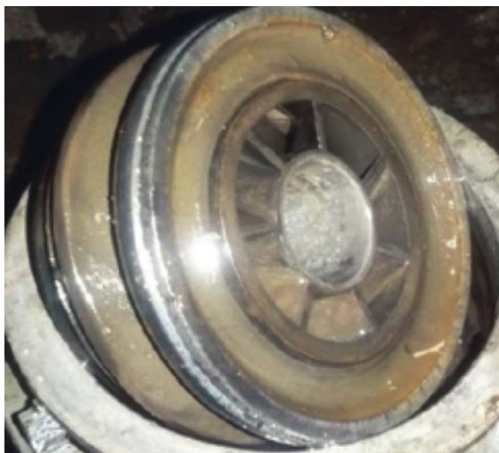
A WR2 Pump Stage after five months of operation in a Permian Basin well shows very little wear from abrasion. (Photo courtesy of Borets)
