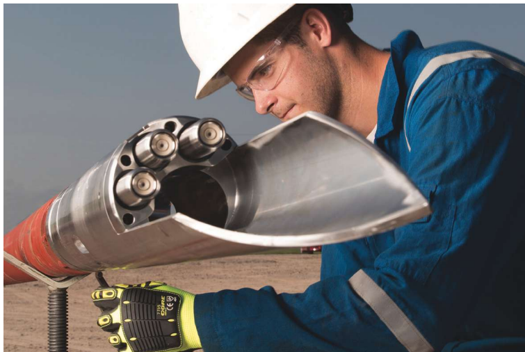
The plug-and-play design of the ZEiTECS Shuttle rigless ESP replacement system enables any standard ESP assembly to be retrieved and redeployed without a rig using wireline, coiled tubing or sucker rods. (Photo courtesy of Schlumberger)
