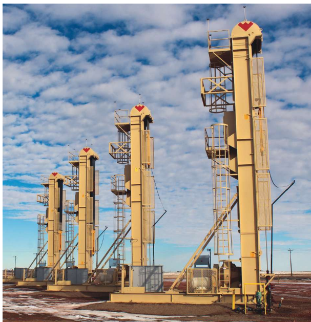
Weatherford's Rotaflex long-stroke pumping units have been successfully installed on wells that produce fluid volumes of up to 1,000 bbl/d. (Photo courtesy of Weatherford)
