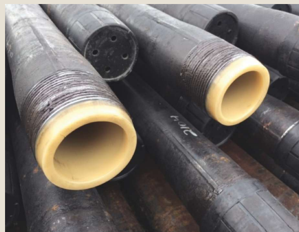
Production tubing is lined with polyolefin ketone thermoplastic liner. (Photo courtesy of Lightning Rod & Pipe)
