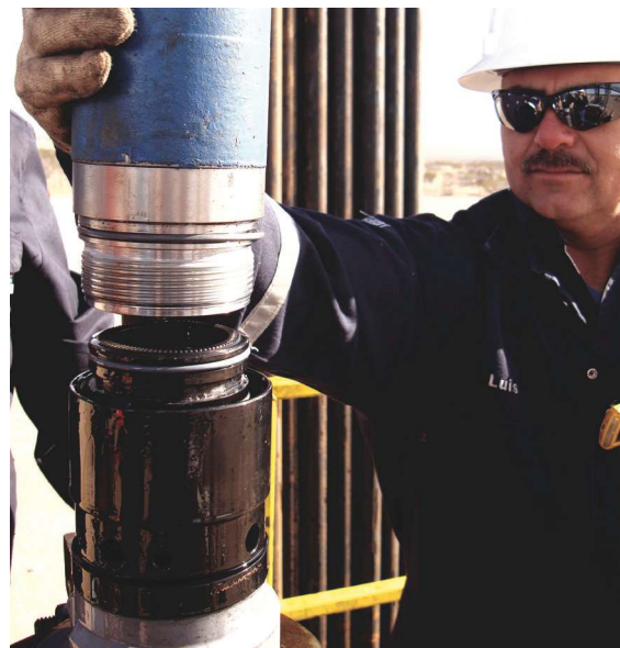
Baker Hughes' CENesis Curve tight-radius production system is designed to pass through a 15-degree per 100-ft bend section in deviated and horizontal wells, allowing operators to land the ESP system closer to the pay zone to maximize production and reserve recovery. (Photo courtesy of Baker Hughes)
