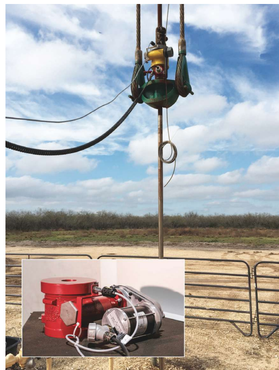
NOV's Smart Rod Rotator (center) automates the routine of checking rod rotator integrity and allows remote monitoring and alarm capabilities. The Hercules ERR (inset) eliminates the need to install a traditional mechanical arm and cable. (Photo courtesy of NOV)
