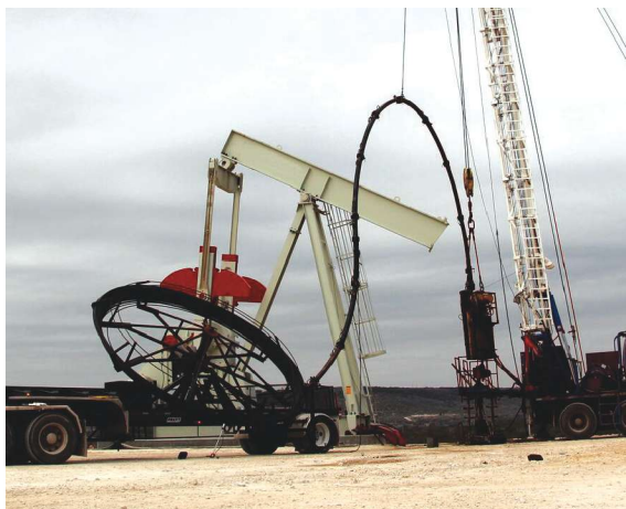
A LightningRod continuous rod installation took place in the Permian Basin, allowing rapid workovers by eliminating the couplings in the rodstring. (Photo courtesy of Lightning Rod and Pipe)
