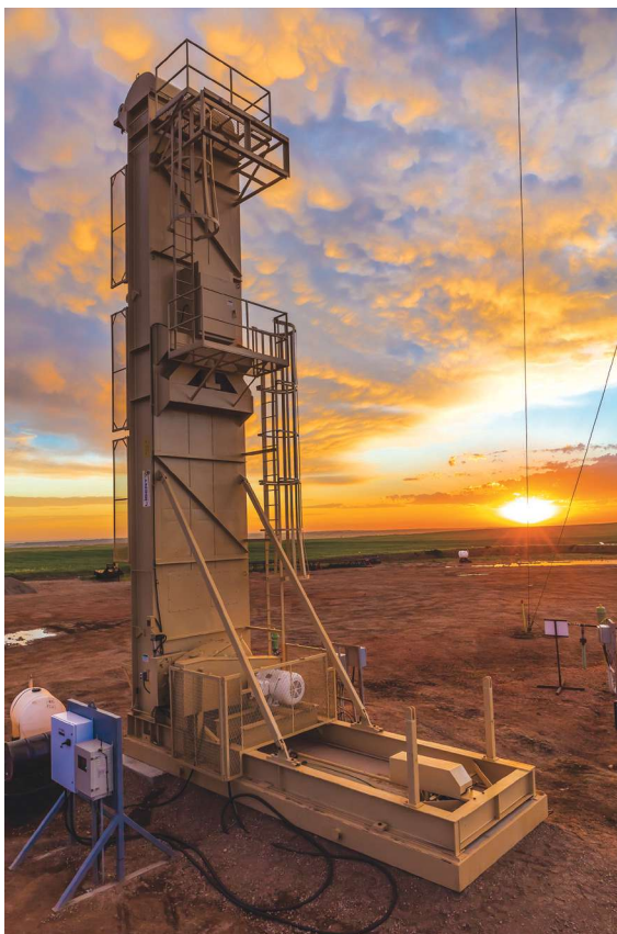
Liberty Lift's XL 366-in. stroke units are well-suited for work in deviated, deep, high-volume wells. (Photo courtesy of Liberty Lift)
