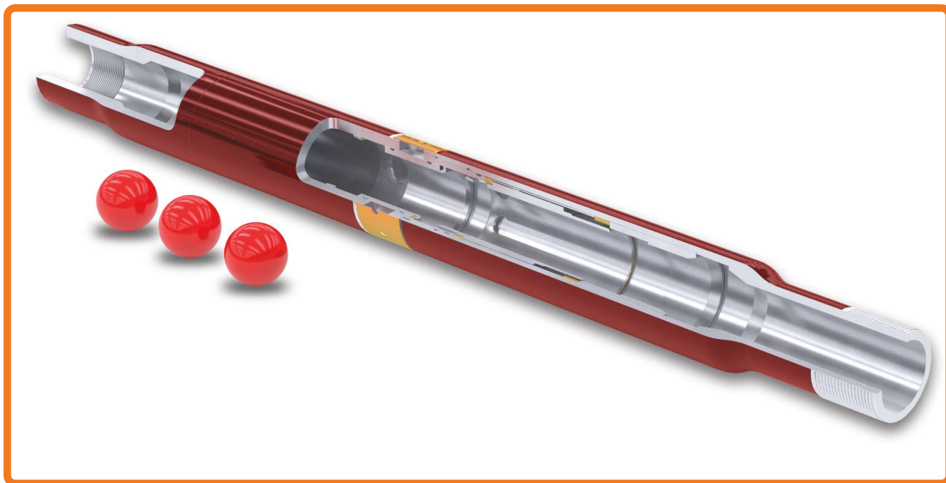
The i-ball technology eliminates downhole pressure buildup and associated logistics and storage concerns by using one ball and one seat size for all sleeves in the lateral casing string. (Image courtesy of Weatherford)
