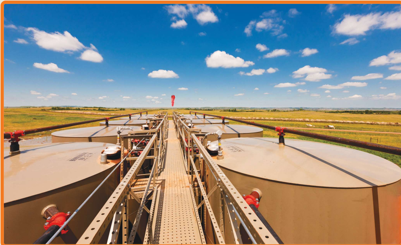
A tank battery gathers Bakken system oil for tank truck pickup in the Williston Basin. (Photo courtesy of Enerplus Corp.)
