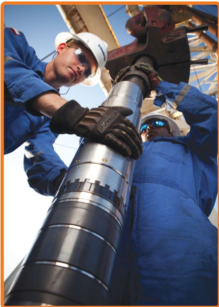
The Falcon multistage stimulation system uses swellable or hydraulically set packers to isolate numerous stages that are then treated continuously. The system is installed in a single trip, reducing rig time, costs, and operational risks. (Image courtesy of Schlumberger)
