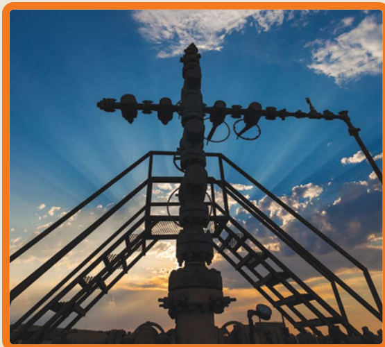
A Williston Basin christmas tree routes production from wells to pipelines and tank batteries. (Photo courtesy of Kodiak Oil & Gas Corp.)
