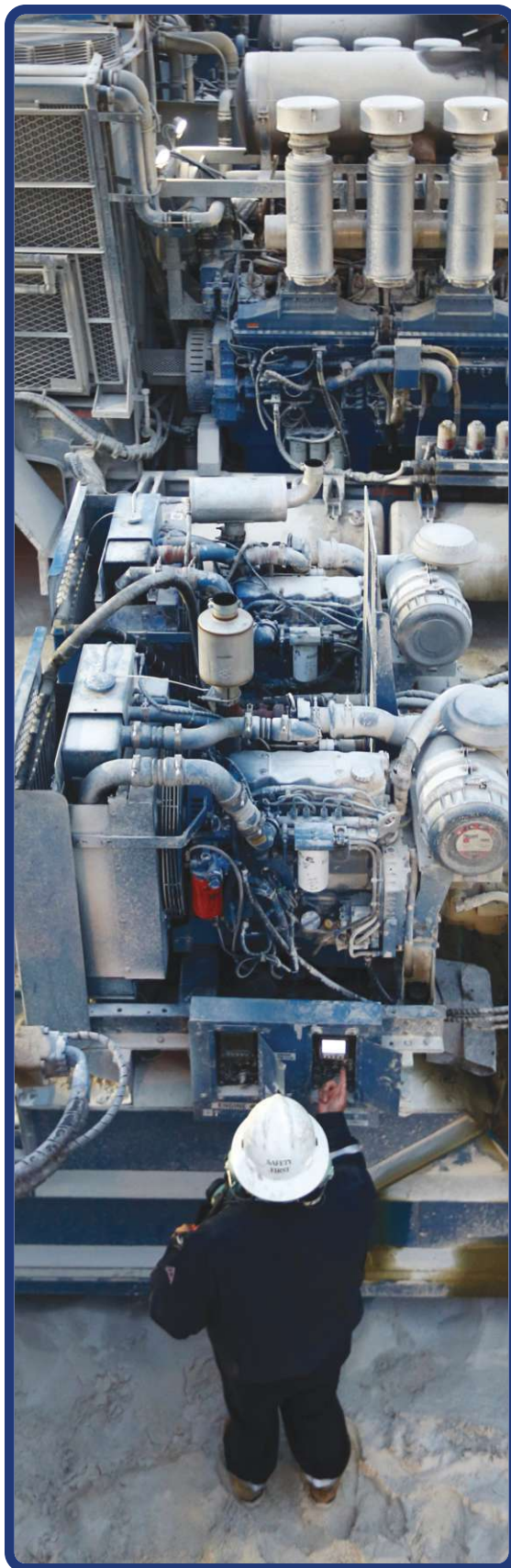
A Baker Hughes crew member monitors propant-mixing equipment on the Gloria Wheeler lease. (Photo by Tom Fox)
