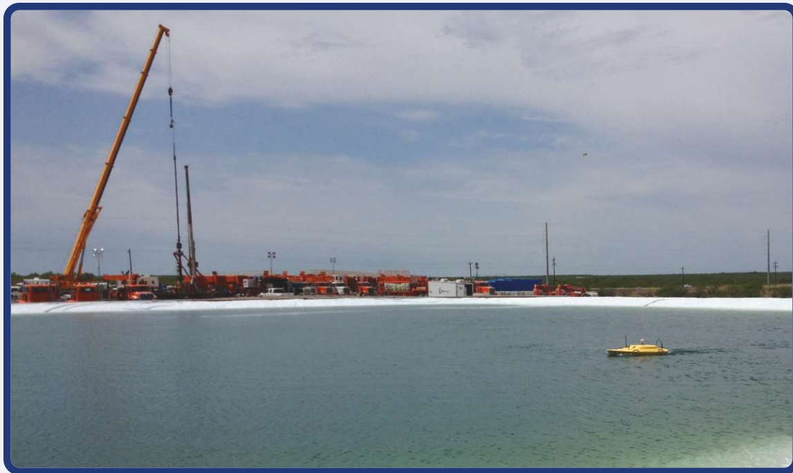
The AquaView boat is shown generating a hydrographic map of a water source in preparation for hydraulic fracturing activity. (Image courtesy of Select Energy Services)
