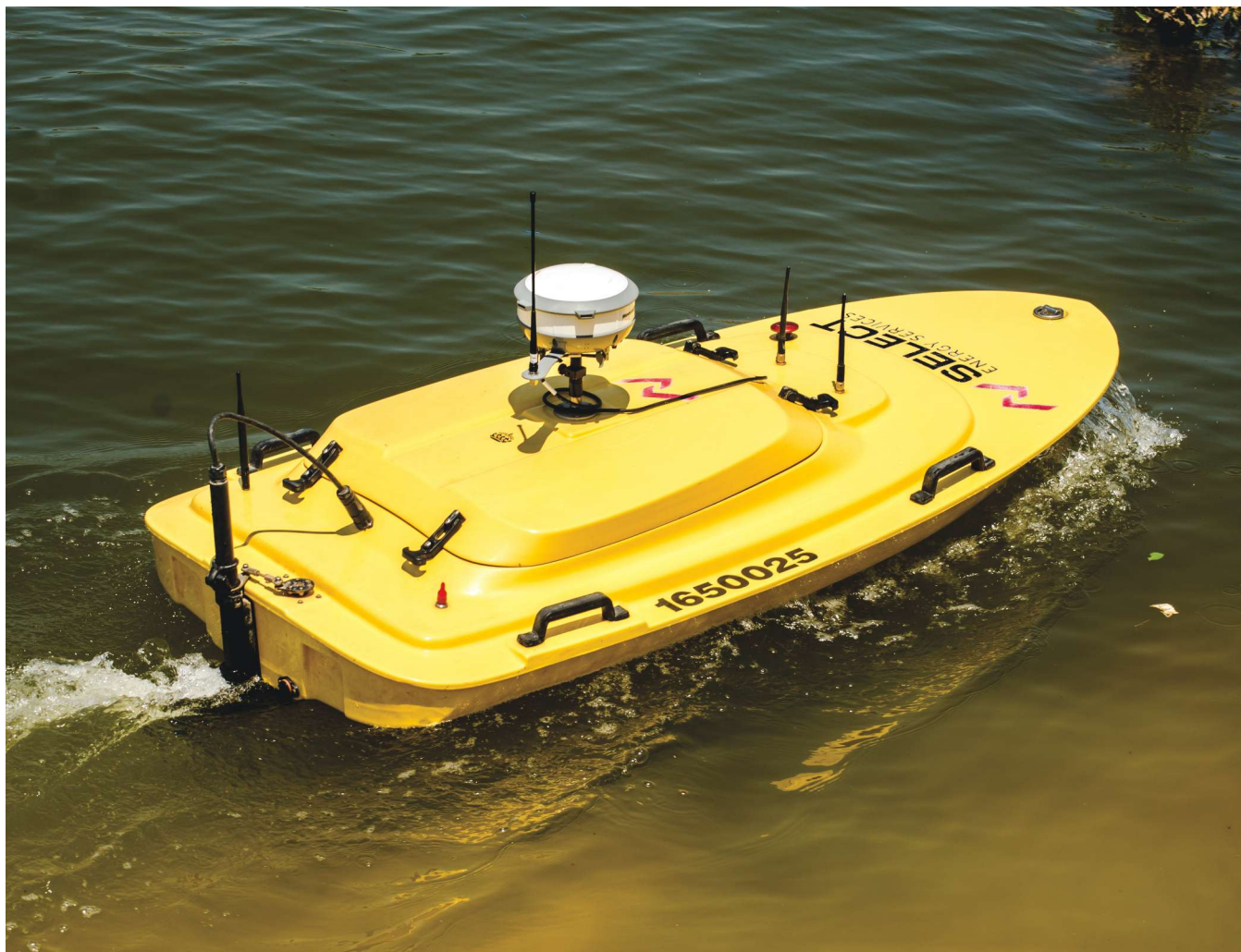
Select Energy Services uses a remote-controlled unit to assist it in data gathering and mapping of water pits as part of its AquaView suite of services. (Image courtesy of Select Energy Services)
