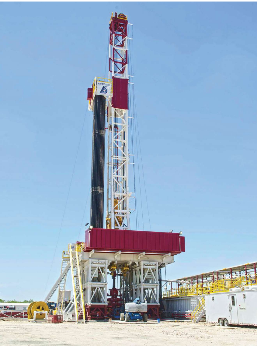
A Sidewinder walking rig drills on a Swift Energy location in the Eagle Ford in McMullen County in South Texas. (Image courtesy of Swift Energy Co.)
