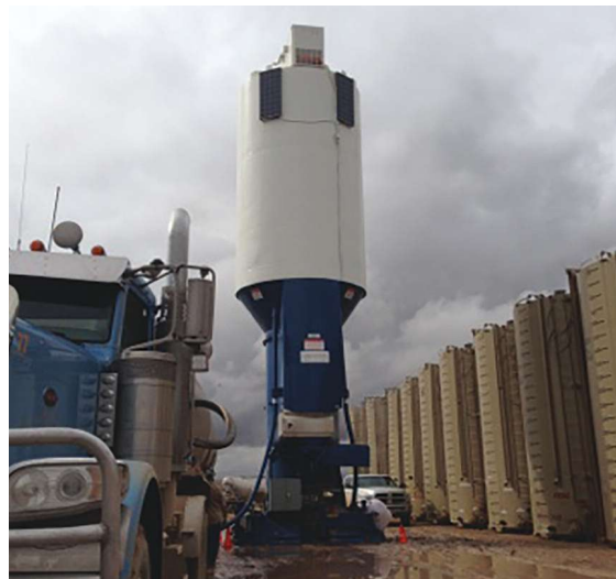
The Quickstand Proppant Silo can be rapidly deployed on site and facilitates large storage of proppant on a smaller footprint. (Image courtesy of Quickthree Solutions)
