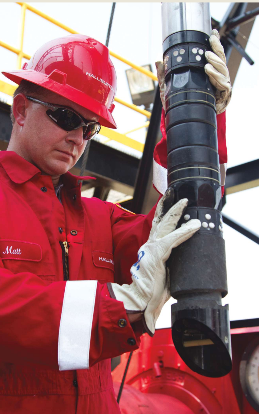
Halliburton Obsidian and Fas Drill composite bridge and frack plugs offer dependable isolation as well as quick and easy removal for a full range of applications. (Image courtesy of Halliburton)
