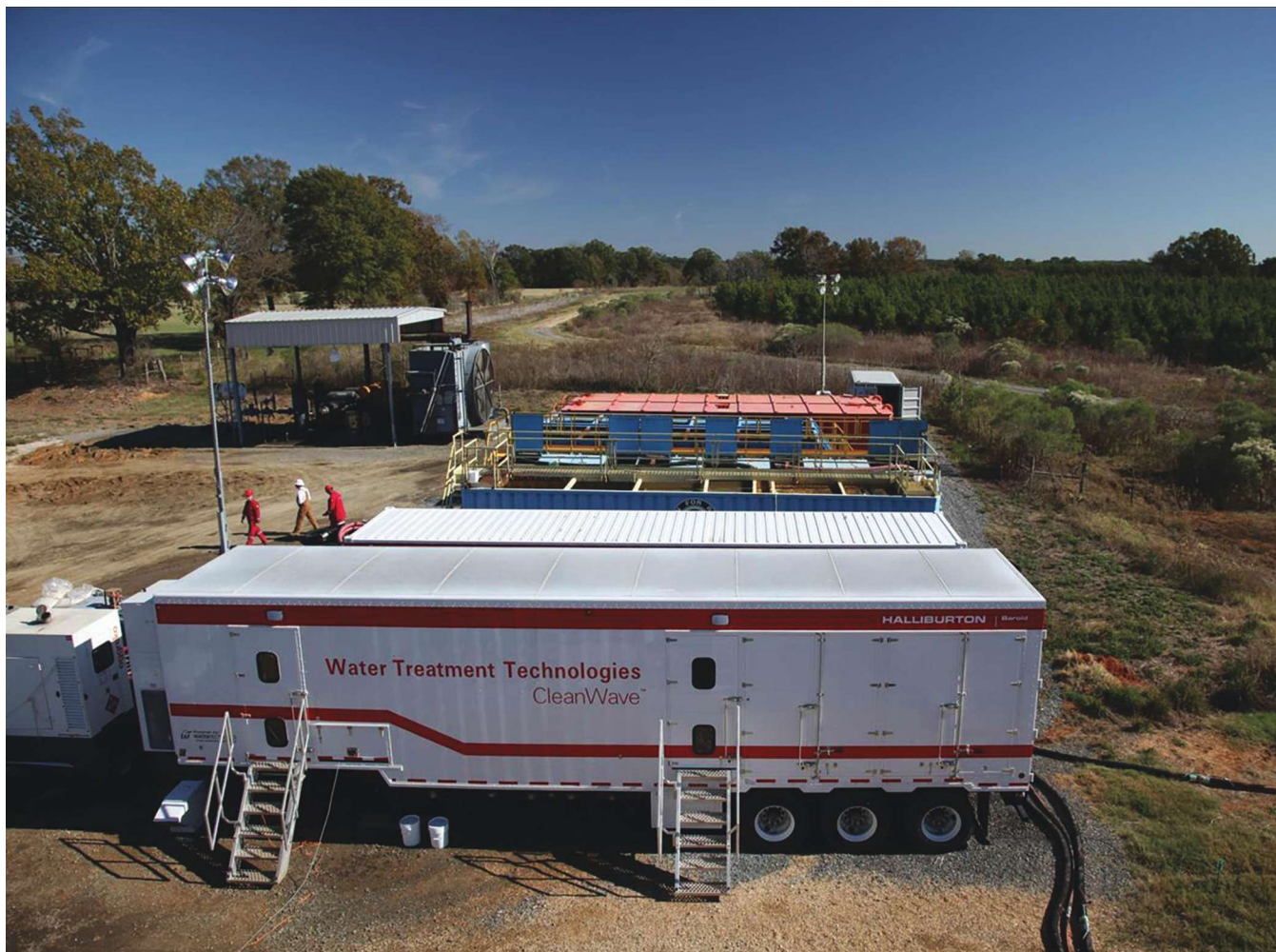
CleanWave destabilizes and coagulates the suspended colloidal matter in water. When contaminated water passes through electro-coagulation cells, the anodic process releases positively charged ions, which bind onto the negatively charged colloidal particles in water resulting in coagulation. (Image courtesy of Halliburton)
