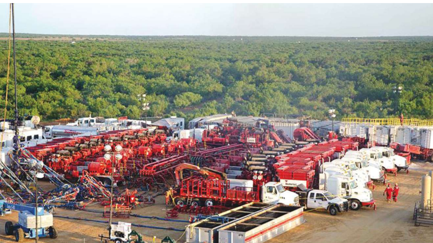
A Weatherford fleet performs hydraulic fracturing on Swift Energy’s Fasken No. 9-H and No. 10-H in Webb County, Texas. (Image courtesy of Swift Energy Co.)
