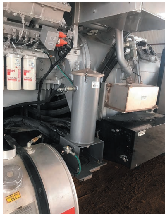
The puraDYN oil bypass filtration system was installed in a fracturing unit. DistributionNOW holds an exclusive global distributorship. (Photo courtesy of Puradyn Filter Technologies Inc.)
