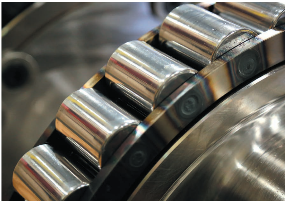
These roller bearings on the QEM 3000 pump follow 2,700 hours of demanding service. (Photo courtesy of Weir Oil & Gas)
