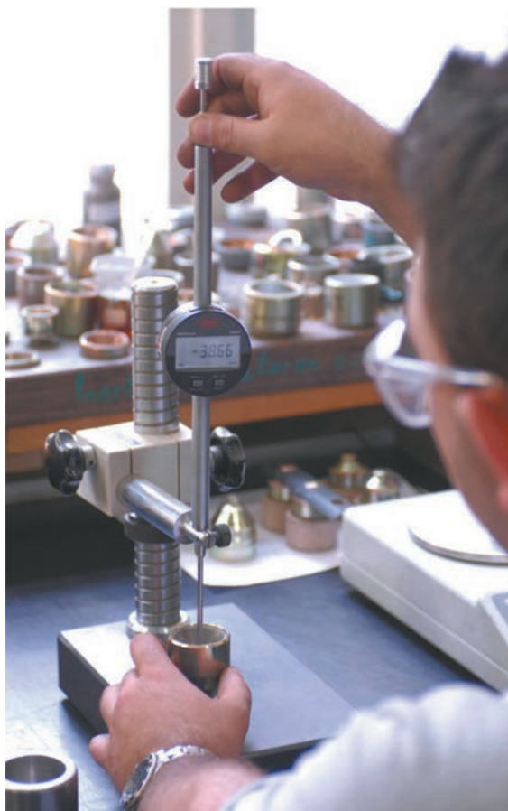
An R&D technician ensures accurate measurements of a shaped charge interior. (Photo courtesy of DynaEnergetics)
