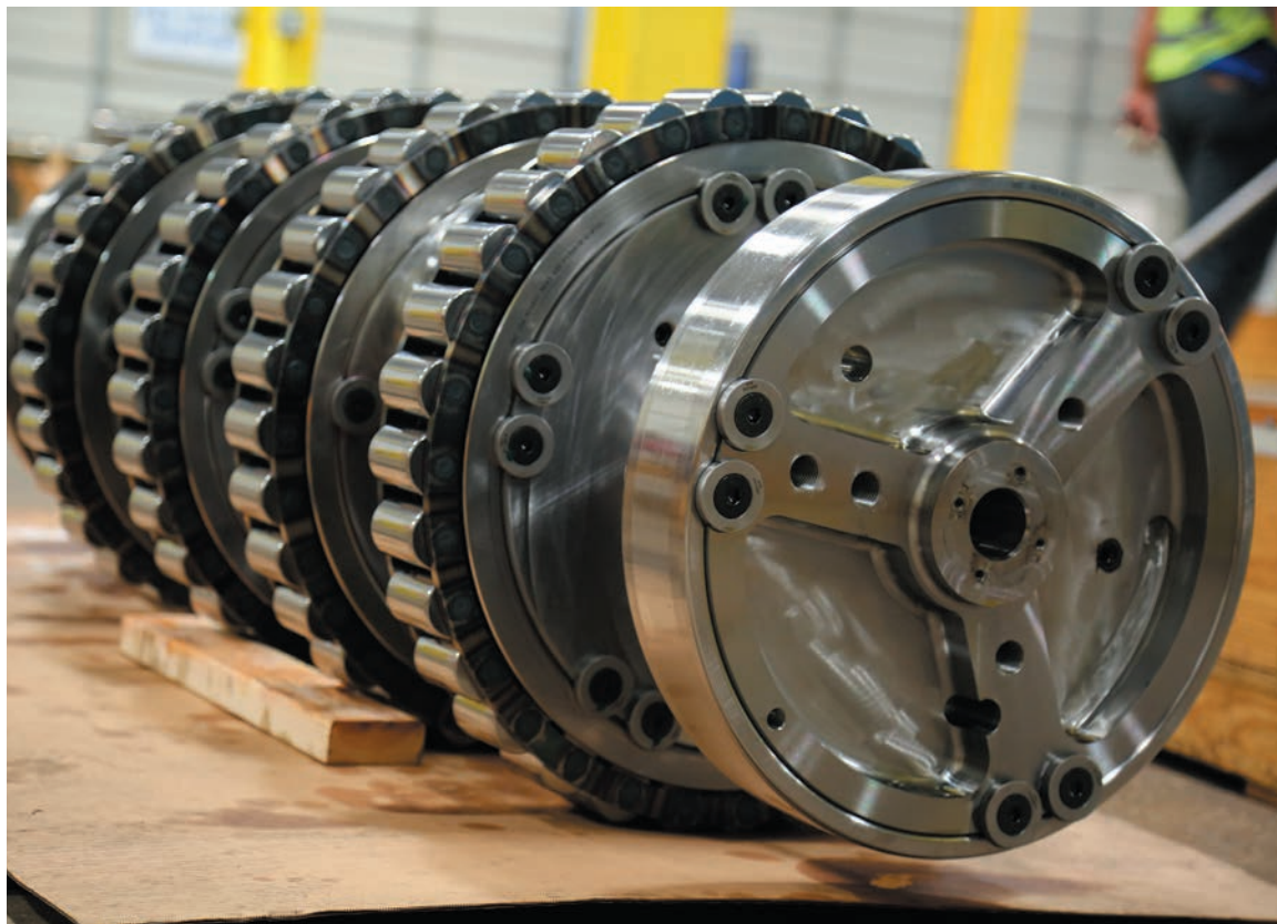
The crank assembly from the QEM 3000 shows minimal wear following 2,700 hours of service. (Photo courtesy of Weir Oil & Gas)
