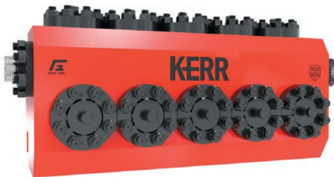
The Kerr Pumps Frac One Connect fluid end bolts right up to existing stay rods with a more rigid flangeless design. It includes replaceable stuffing box sleeves with all seals embedded into the fluid end to prevent washouts. (Image courtesy of Kerr)
