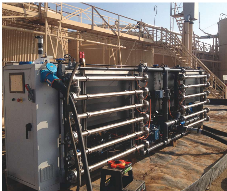
OriginClear's 3,000-bbl/d EWS test unit is shown at a produced water site in the Monterey Formation. (Image courtesy of OriginClear)
