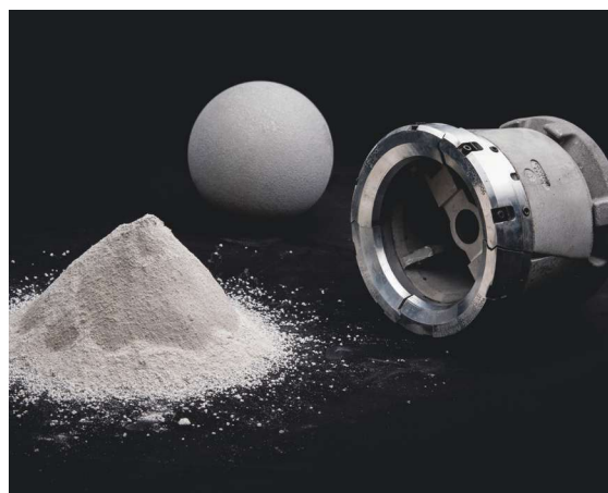
The degradable fracture ball and seat dissolve completely, eliminating the need for milling and enabling fullbore production. (Image courtesy of Schlumberger)
