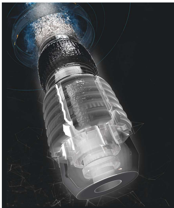
The Baker Hughes dissolvable frack plug uses CEM nanostructured material that enables the plug body, anchoring grip and packing element to disintegrate completely downhole when in contact with produced fluids. (Image courtesy of Baker Hughes)
