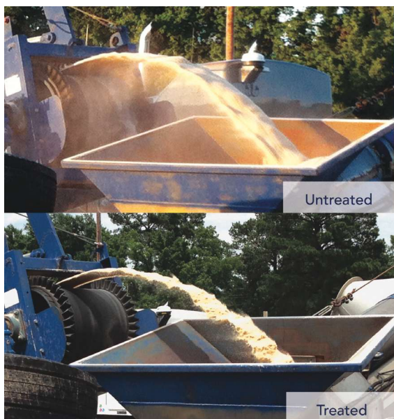
This comparison shows untreated fracture sand vs. fracture sand treated with SandTec. (Photos courtesy of ArrMaz)
