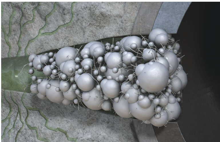
OpenPath Sequence diversion stimulation service uses the optimal acid identified for a particular reservoir to sequentially stimulate targeted zones and intervals. (Image courtesy of Schlumberger)
