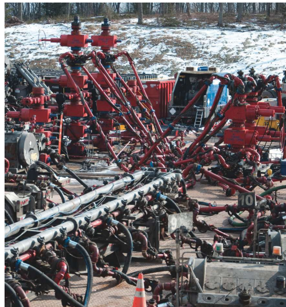
Universal Pressure Pumping fracturing equipment is rigged up on location in Appalachia. (Photo courtesy of Universal Pressure Pumping)
