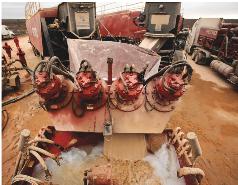
Sand is mixed in with water during fracturing operations for use in a Permian Basin oil well. (Photo by Tom Fox, courtesy of Oil and Gas Investor)
