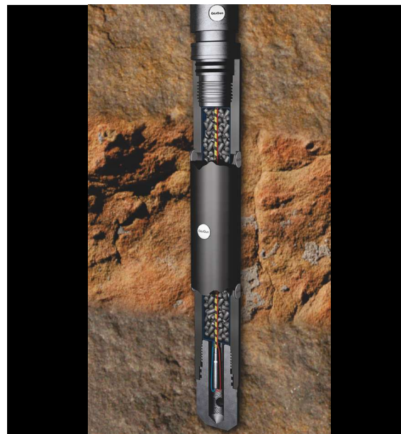
The GasGun propellant fracturing stimulation device installed in Canada was designed to create fractures and increase formation permeability. (Image courtesy of GasGun)
