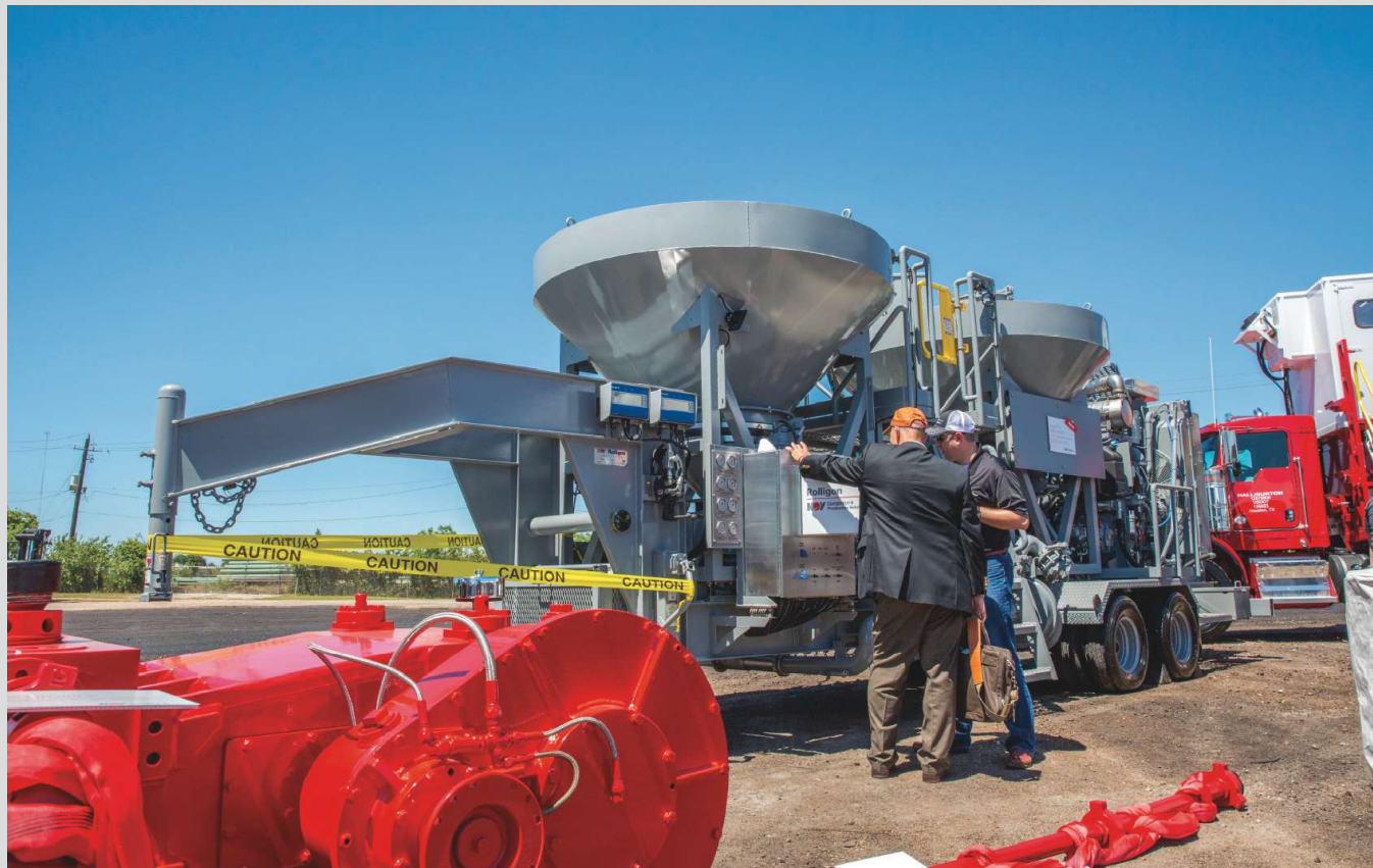
The dry additive mixing unit uses a custom-designed mixer to pre-mix the gel powder with water onsite. (Photo courtesy of NOV)
