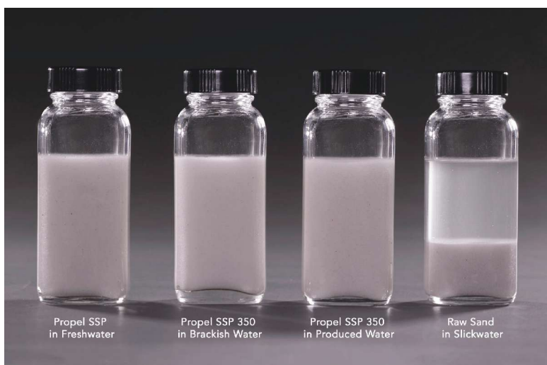
Propel SSP proppant transport technology swells and self suspends in water up to 350,000 ppm TDS, maximizing the effective propped area. (Photo courtesy of Fairmount Santrol)
