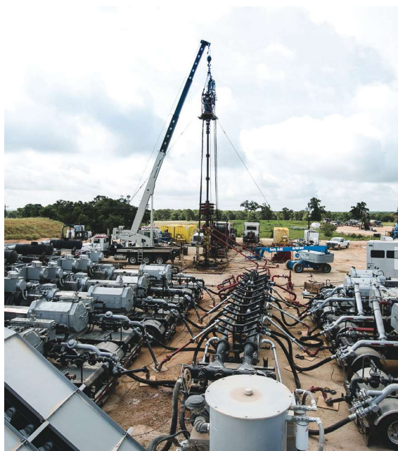
In July Legend Energy Services was operating a CT site in the Eagle Ford in Milano, Texas. The 75,000-hp fleet, built by NOV in the first quarter, comprises fracturing pumps, sanders and unloaders, multisanders, hydration systems, blenders, and liquid additive systems. (Photo courtesy of NOV)
