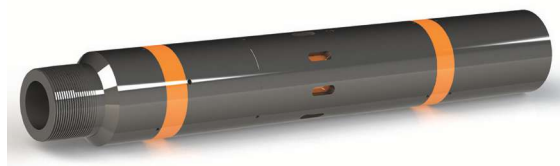
The PosiFrac Toe Sleeve assembly is designed for cemented or uncemented completions where a casing pressure test is desired to confirm casing integrity prior to opening the toe sleeve. (Image courtesy of Tam International)
