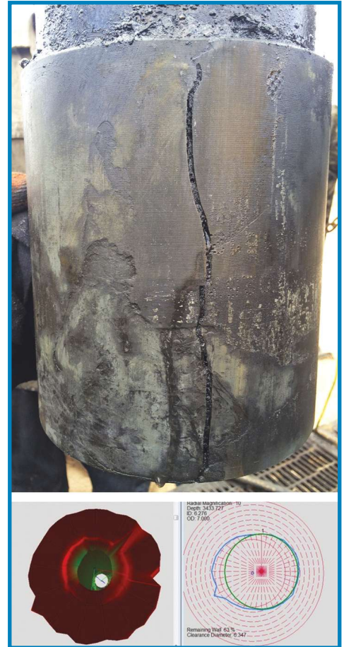
The Weatherford SecureView service provided an exact cased-hole evaluation for a leaking well in the Wolfcamp Shale. The pulled casing (top) shows damage identical to the damage indicated by the logs (bottom). (Image courtesy of Weatherford)
