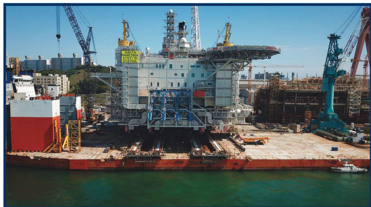
Statoil's Aasta Hansteen topside is loaded out on the Dockwise White Marlin heavy-transport vessel at Hyundai Heavy Industries en route to Norway. This will be the first spar offshore Norway and the largest in the world. (Photo by Lee Hyungjin, courtesy of Statoil)
