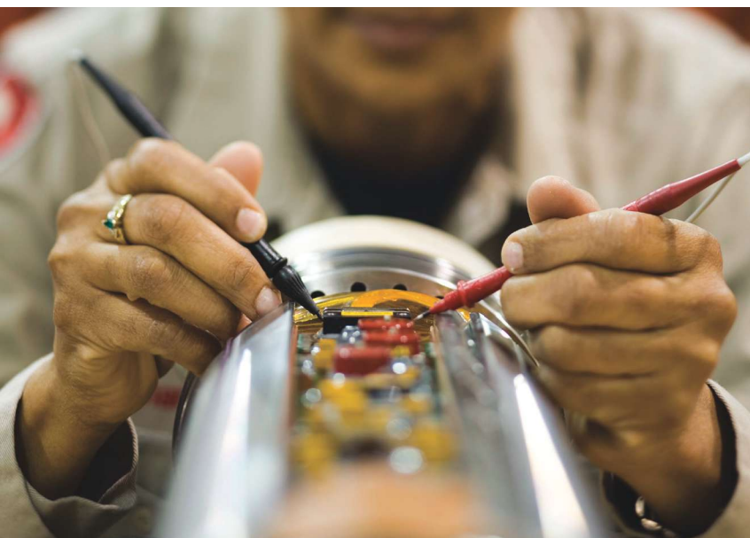
The Extreme HeatWave HP/HT LWD tool has a temperature rating of 200 C and a pressure rating of 30,000 psi. Data can be recorded at ROPs up to 720 ft/hr. (Image courtesy of Weatherford)
