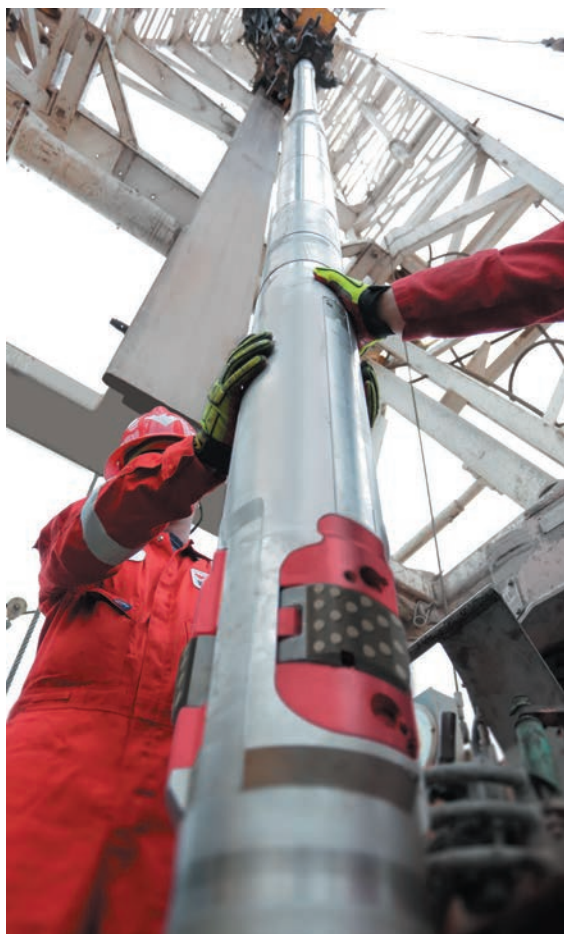
The Magnus RSS improves directional control when drilling in tight target windows. (Photo courtesy of Weatherford)
