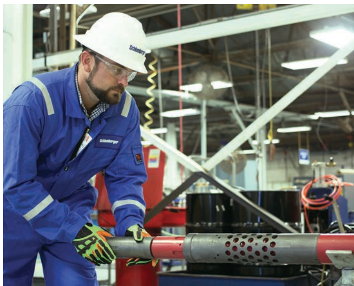
The HEAL system—which separates the horizontal from the vertical well sections and regulates the flow between them—has no moving parts and can be connected to any variant of lift system. (Photo courtesy of Schlumberger)
