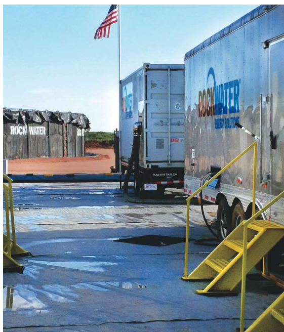
Oilfield water treatment can involve any number of technologies depending on the incoming water conditions—from filtration to electro-oxidation, which is used on this location in Pecos, Texas, by Rockwater. (Photo courtesy of Rockwater Energy Solutions)
