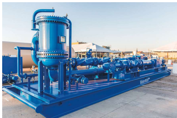
The WaterWolf DOR 500 can handle up to 50,000 bbl/d of water. (Photo courtesy of NOV)
