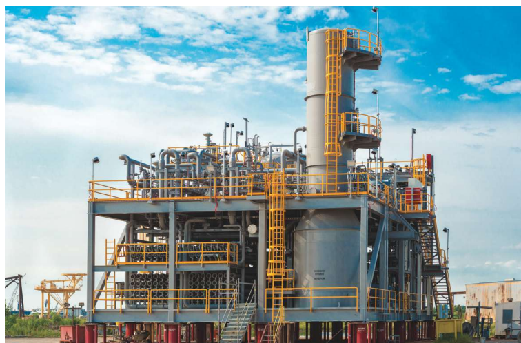
The Schlumberger seawater injection module treats the seawater for reinjection in the secondary and tertiary oil recovery cycles. (Image courtesy of Schlumberger)
