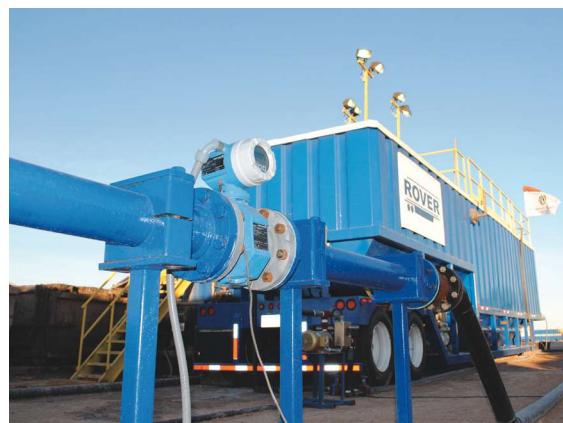
ROVER technology removes suspended solids and polymers and is capable of recycling 10,000 bbl/d of clean brine. (Photo courtesy of Fountain Quail Energy Services)
