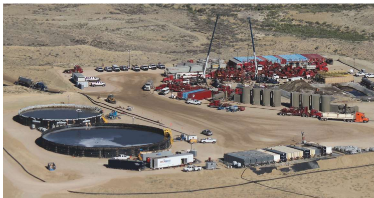
Rockwater fluids conditioning setup taps into a customer's produced water gathering system, centralizing water treatment for reuse on multiple fractures in the Rockies. (Photo courtesy of Rockwater Energy Solutions)
