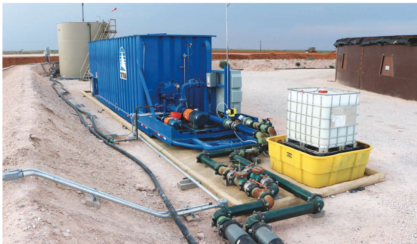
With potential throughput ranging from 25,000 to 35,000 bbl/d, the TETRA ORAPT helps pull out as much oil as possible prior to filtering and blending produced water—down to 50 to 100 parts per million. (Photo courtesy of TETRA Technologies Inc.)
