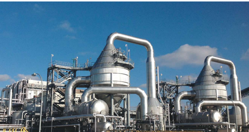
Veolia's CoLD crystallization is applied to produced water with very high TDS to increase water recovery. (Photo courtesy of Veolia Water Technologies)
