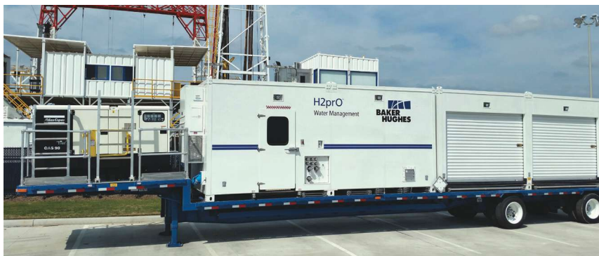
The H2prO SR water management service uses proven filtration technology in a highly mobile system to remove suspended solids from produced and flowback water. (Photo courtesy of Baker Hughes)
