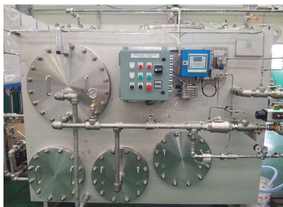
The Crystal separators have a filter-less operation with no internal moving parts. (Photo courtesy of GenOil)
