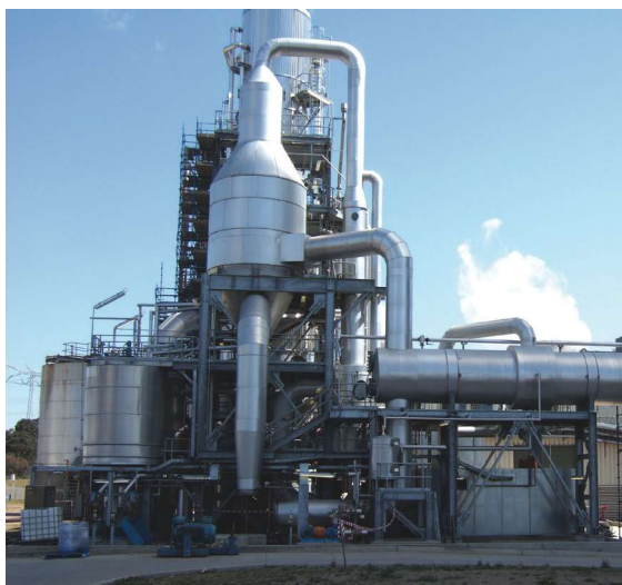
Veolia's MBD (modular bulldozer design) evaporation/crystallization system is designed to reduce installation time and cost. (Photo courtesy of Veolia)
