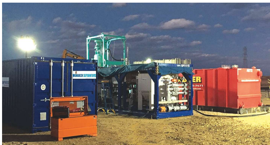
The mobile produced and flowback water treatment system is operating to treat water for reuse in fracturing operations and to meet stringent regulations for safe discharge into a nearby river. The system is designed to remove total suspended solids, benzene, toluene, ethylbenzene and xylene, oil, iron, manganese, H 2 S and ammonia. (Photo courtesy of Water Standard)
