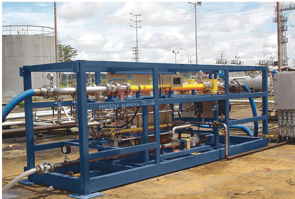
Voraxial impeller-induced cyclonics provide a robust, flexible, onsite separation method in a compact, self-contained unit for high-rate water treatment. (Photo courtesy of Schlumberger)
