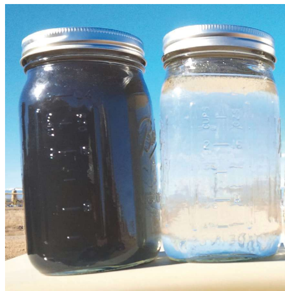
A blend of produced and flowback water undergo treatment via Water Standard’s mobile system. These water samples demonstrate the before and after treatment. (Photo courtesy of Water Standard)
