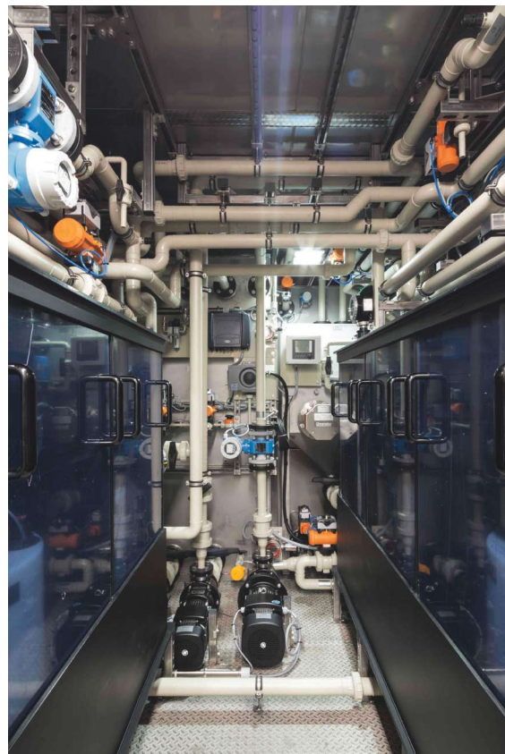
This detailed view shows the ultrafiltration module and piping in OilPaq’s container. (Photo courtesy of APATEQ)
