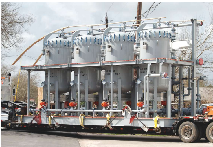
A produced water treatment skid leaving Water Standard's Monarch fabrication facility was headed to an offshore platform in the Gulf of Mexico. (Photo courtesy of Water Standard)
