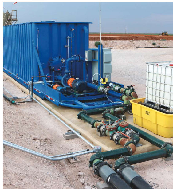
With potential throughput ranging from 25,000 bbl/d to 35,000 bbl/d, the TETRA Orapt helps pull out as much oil as possible prior to filtering and blending produced water—down to 50 ppm to 100 ppm. (Photo courtesy of TETRA Technologies Inc.)
