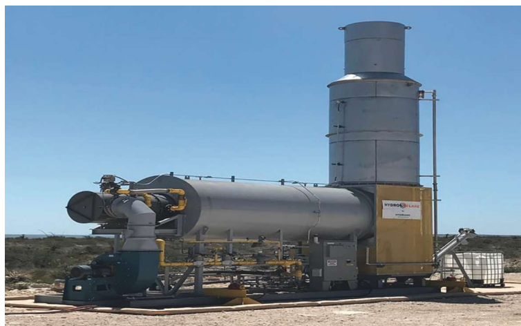
The HydroFlare system is in the field in the Permian Basin awaiting commissioning. The system essentially converts the flare into an evaporator. (Photo courtesy of Hydrozonix)
