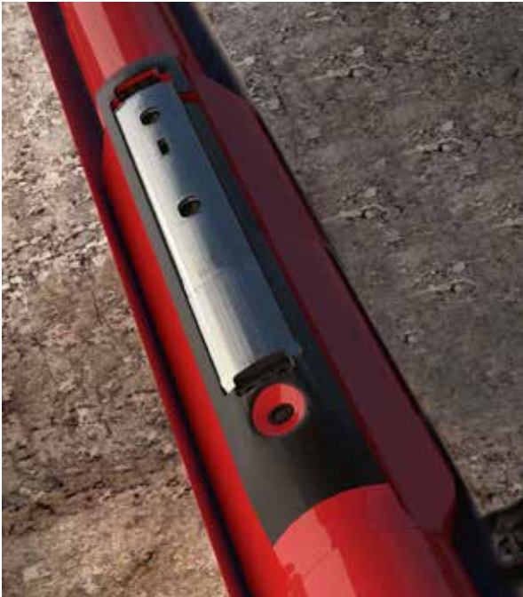
The ALD LWD Service reduces geological uncertainty and refines the earth model by measuring structural dip in real time. (Image courtesy of Halliburton)
