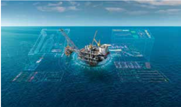
Digital twins are dynamic, cross-domain digital models that mirror the performance and operation of a physical asset or process as it moves through the life cycle. (Image courtesy of Siemens)
