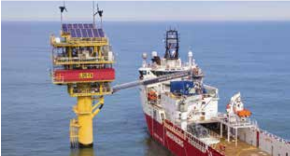
Ampelmann’s A EP gangway system will transfer personnel from Wagenborg Offshore’s second W2W ERRV Kasteelborg to support gas production in the Dutch and U.K. sectors of the southern North Sea. (Photo courtesy of Ampelmann)
