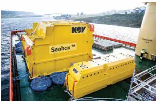
The Seabox subsea water treatment module takes water treatment from topside to the seabed. (Photo courtesy of National Oilwell Varco)
