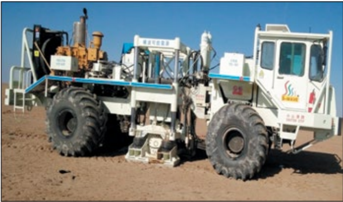
FIGURE 1. BGP upgraded a high tonnage shear-wave vibrator (DV300S). (Images courtesy of BGP)
